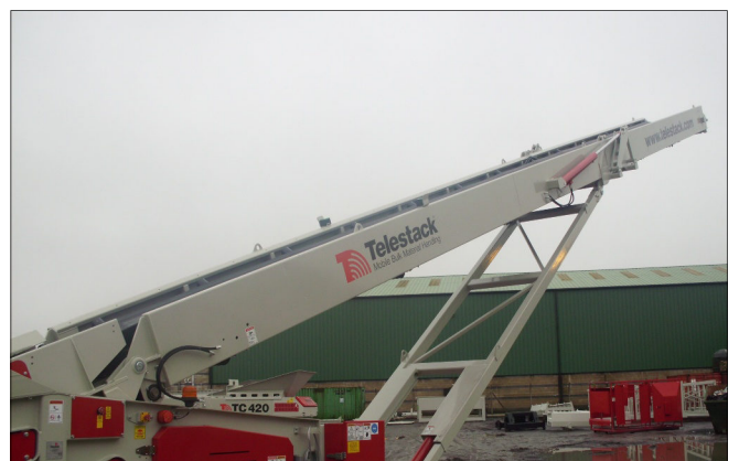
Heavy duty - 18 metre (60ft) Incline conveyor
