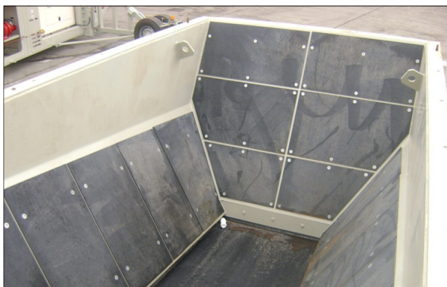
Hopper with optional bolt-in liners
