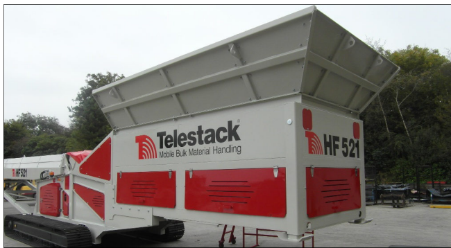
7m 3 Hopper - Optional 9m 3 and 12m 3 Upgrades
