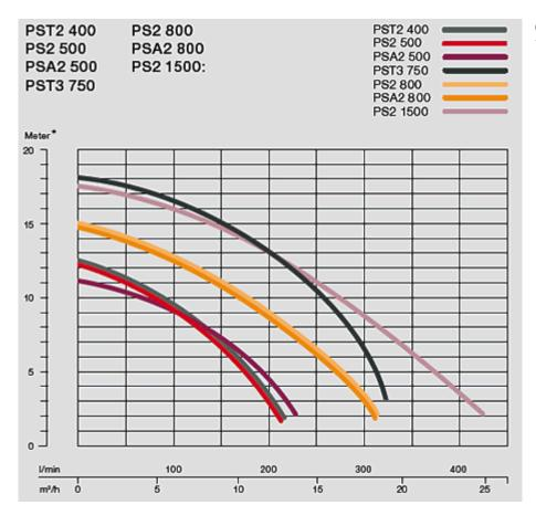
Operation at 3,500 1/min \* total discharge head
